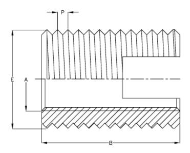
Female thread A = M8Length B = 12Male thread E = 10.0Min hole depth blind hole = 15Recommended bore diameter (hard mat.) = 8.9 to 9.2Recommended bore diameter (soft mat.) = 8.6 to 8.8Thread pitch P = 1.00Type  $= 303 \ 0 \ 080$ ..
